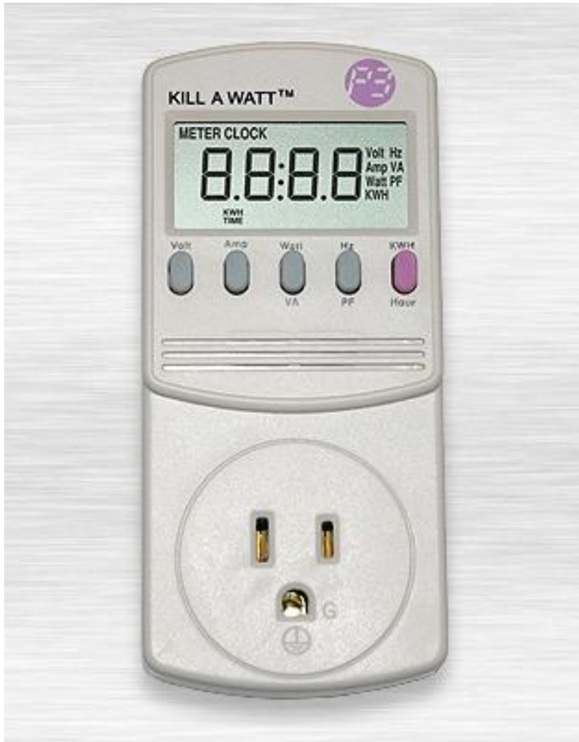
Figure A1 Killawatt Meter (Source: Iona Lake Electricity Corp)
